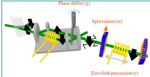
$$|\Psi_{\text{Neutron}}\rangle = \left( |\Psi_I\rangle \otimes |\uparrow\rangle \otimes |\Psi(E_0)\rangle \right) + \left( e^{i\chi} |\Psi_{II}\rangle \right) \otimes \left( e^{i\alpha} |\downarrow\rangle \right) \otimes \left( e^{i\gamma} |\Psi(E_0 + \hbar\omega_r)\rangle \right)$$
