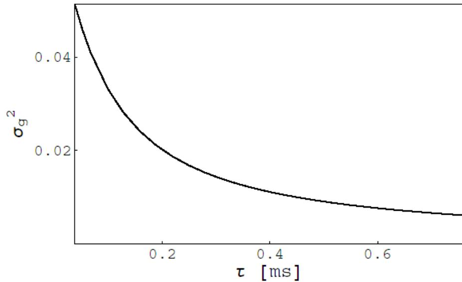
Variance of geometric phase ( $\sigma_g^2$ ) tends to 0 for increasing time of evolution in a magnetic field.
