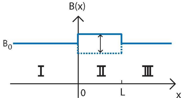
$$i\hbar \frac{\partial \psi(\vec{r},t)}{\partial t} = H\psi(\vec{r},t) = \left( \frac{\hbar^2 k^2}{2m} + \mu\hat{\sigma}B(\vec{r},t) \right)\psi(\vec{r},t)$$
