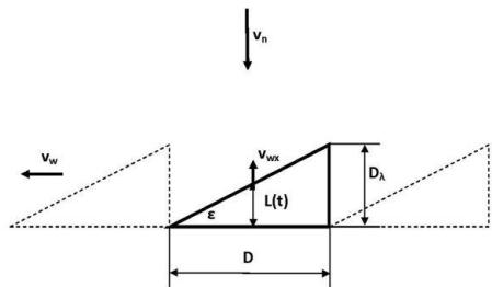
$$x \equiv L(t) = D_\lambda v_w t / D = v_w t \tan \alpha; \quad D_\lambda = 2\pi / Nb_c \lambda$$
