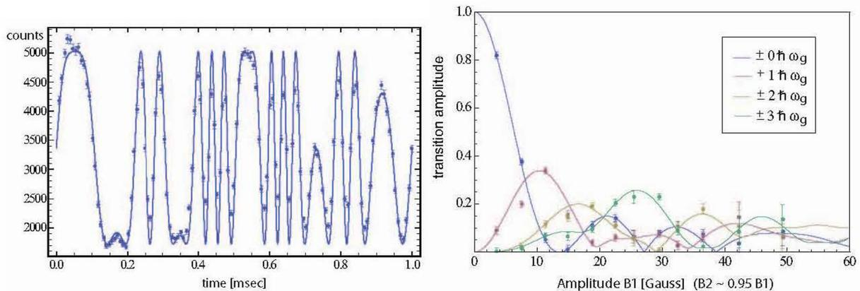
**Figure 6.** Example of a time-resolved interference pattern for a two mode field  $f_1 = 3\text{kHz}$  and  $f_2 = 3\text{kHz}$  and  $B_1 = 30\text{ G}$  (left) and extracted multi-photon transition probabilities (right) (Sulyok et al. [15])
