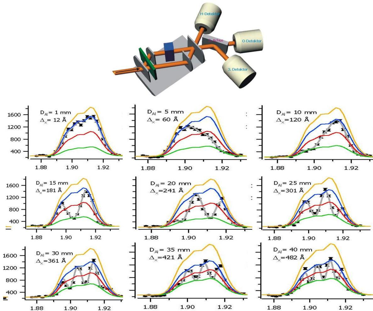
**Figure 2.** Experimental arrangement (top) with a third crystal as a momentum (wavelength) filter and typical momentum scans at different interference order (Baron and Rauch [8])
