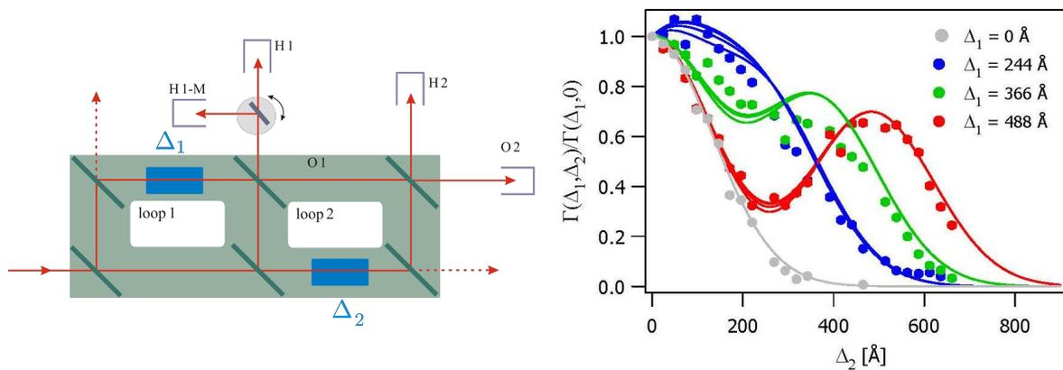
**Figure 3.** Double loop interferometer (left) and measured spatial distribution for different phase shifts in the first loop (Baron and Rauch [8])
