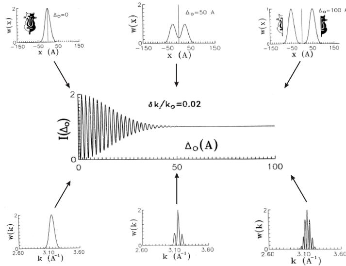
**Figure 1.** Wave packets and momentum distributions for various phase shifts at low and high interference order (Rauch [6])
