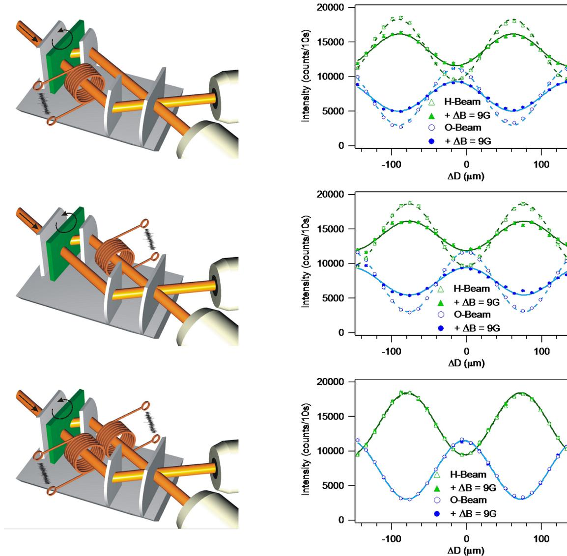
**Figure 4.** Interference pattern with (full lines) and without magnetic noise field (dashed lines) with frequencies between 0 and 20kHz and a mean amplitude of 9 G (Baron and Rauch [8]). The noise field has been applied to the beams separately (top and middle) and to both beams synchronously (bottom).
